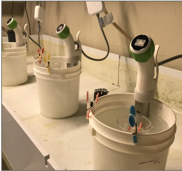
Three temperature treatment baths at 22°C, 25°C, and 28°C
